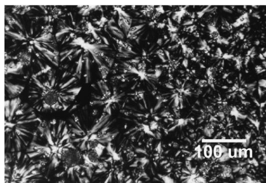
Fig. 4. Polarised light microphotographs after isothermal crystallisation at 125 °C of the: (a) pure iPP, (b) PP/Vectra (99/1) blend and (c) PP/Vectra (95/5) blend.
